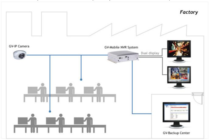
The GV-FER521 and GV-MDR120 / 220 / 320 / 520 / 1500 Series are complied with EN50155 and suitable for the installation with GV-Mobile NVR System. With a mobile device or an Internet browser, you can access the live view and recorded events anywhere.
