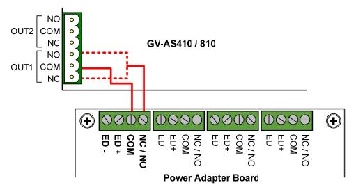
2. Connect the **ED + / -** pins to the (+) and (-) points on the output device (ex: electric lock).
