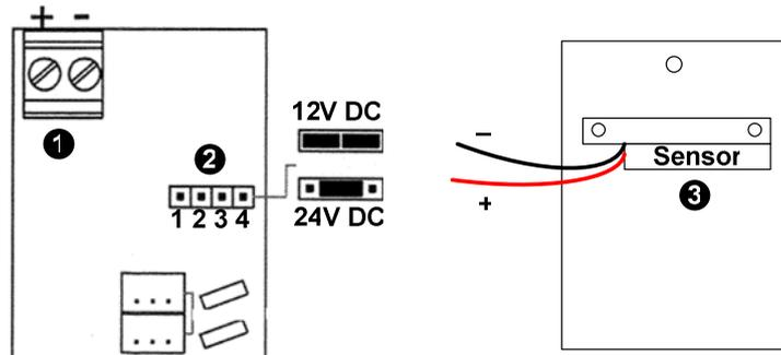
1. **Power Terminal Block:** Connects to the DC 12V / 24V power source.
