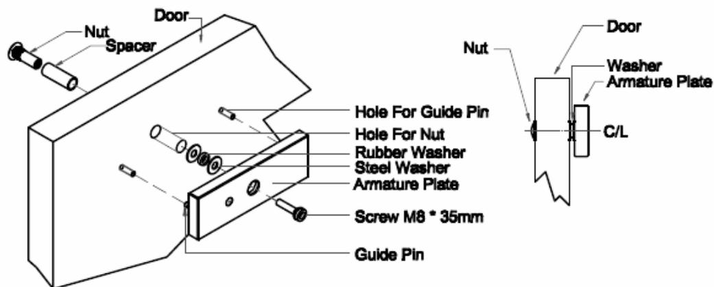
Typical Installation of the electromagnetic lock:
