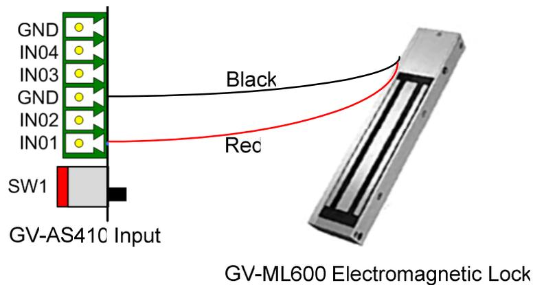
2. On the Web interface of the GV-AS410, select **Input Configuration** under **Advanced Setting**, and select an input type and input function for the connected sensor from the electromagnetic lock.
