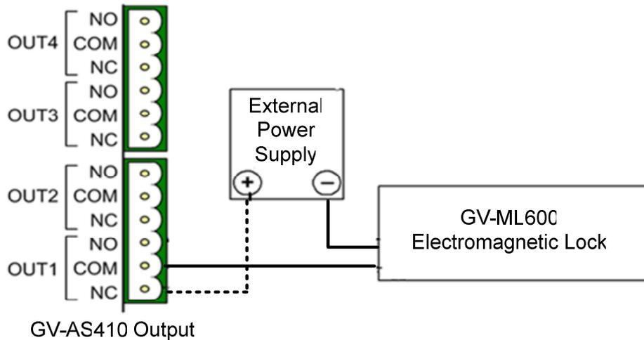
Connect the (+) point on the electromagnetic lock to **COM** on GV-AS410, connect the two (-) points of the electromagnetic lock and the external power supply together, and connect the (+) point on the external power supply to **NC** on GV-AS410.
