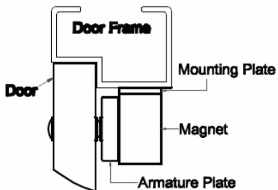
**Note:** To make the armature plate adjust its proper position to the magnet automatically, do not fix the armature plate too tightly and make the rubber washer more flexible.
