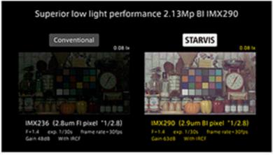
The sensor is designed for security camera to capture usable images even at extremely low-light environment.
